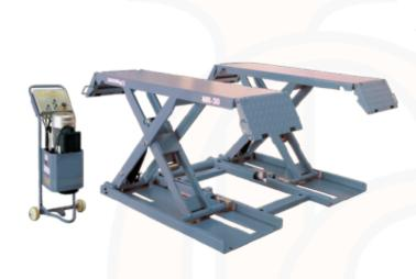
The MR30's one meter lifting height makes it comfortable for tyre, brake, suspension, paint and other bodywork tasks. With its elaborate design, reasonable structure and easily operation, it is very popular with customers. When using this hoist, the bottom frame could be placed on the ground or embedded below the ground. These two bottom frames must be on a level floor, and can be fixed to the ground with anchor bolts.
